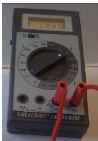
*Figure 8.1: Simple multimeter*
