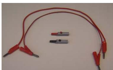
*Figure 8.2: Experimental cables and crocodile clips*
