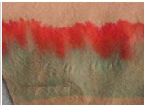
*Figure 10.4: Chromatogram of a brown felt tip*
