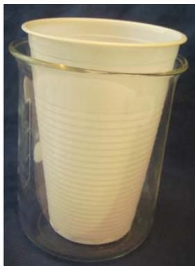
*Figure 9.3: Low cost calorimeter*
