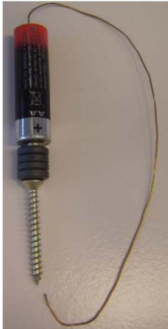
*Figure 8.5: Self constructed electric motor*
