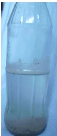
*Figure 7.6: Limewater made from rapid-hardening cement*
