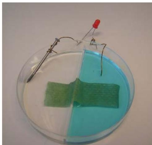
*Figure 8.8: Daniell element with LED for power verification*
