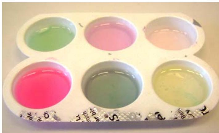
*Figure 10.6: Color scale of red cabbage indicator in a variety of solutions from the household*
