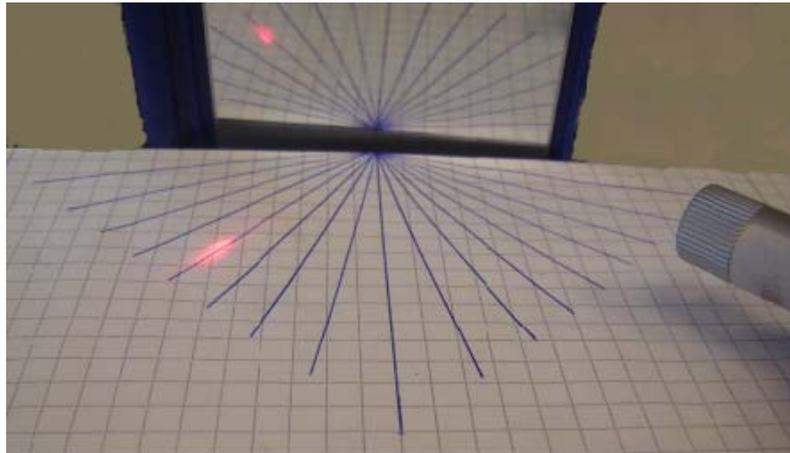
*Figure 8.7: Experiment on the law of reflections*
