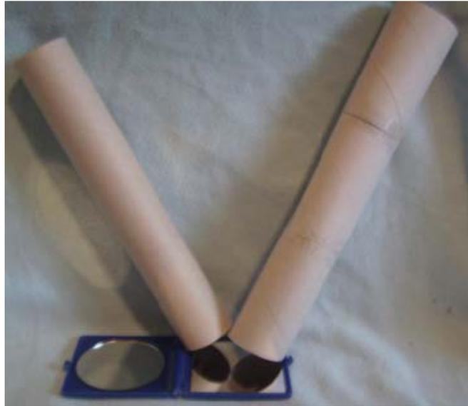
*Figure 7.4: Experiment on the law of reflection*
