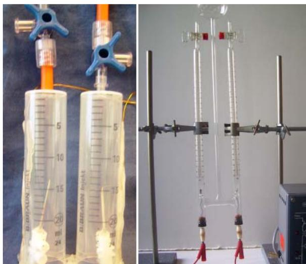
*Figure 3.5: Comparison of an instrument by Hoffmann made of medical engineered elements and one made of glass.*
