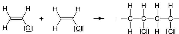
Reaction of vinyl chlorid to polyvinyl chlorid
